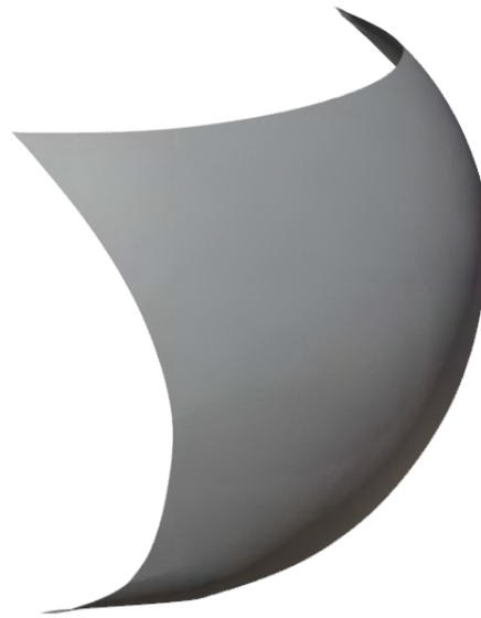
Figure 7.2: Reconstructed model of the surface of the tin sphere acquired at 20 keV, 14mm and 1,1nA.
