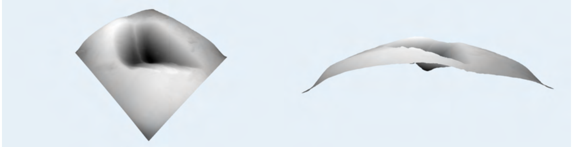
Figure 4.6: 3D model of a ridge in an indium wire reconstructed by Point Electronic microShape.
