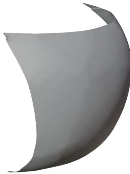
Figure 7.5: Reconstructed model of the surface of the tin sphere acquired at 30 keV, 20mm and 0,9nA.
