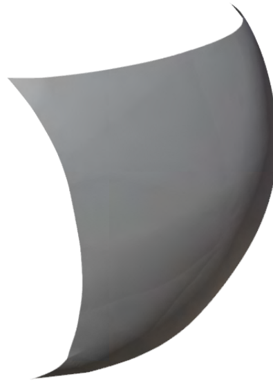
Figure 7.8: Reconstructed model of the surface of the tin sphere acquired at 5 keV, 12mm and 10nA.
