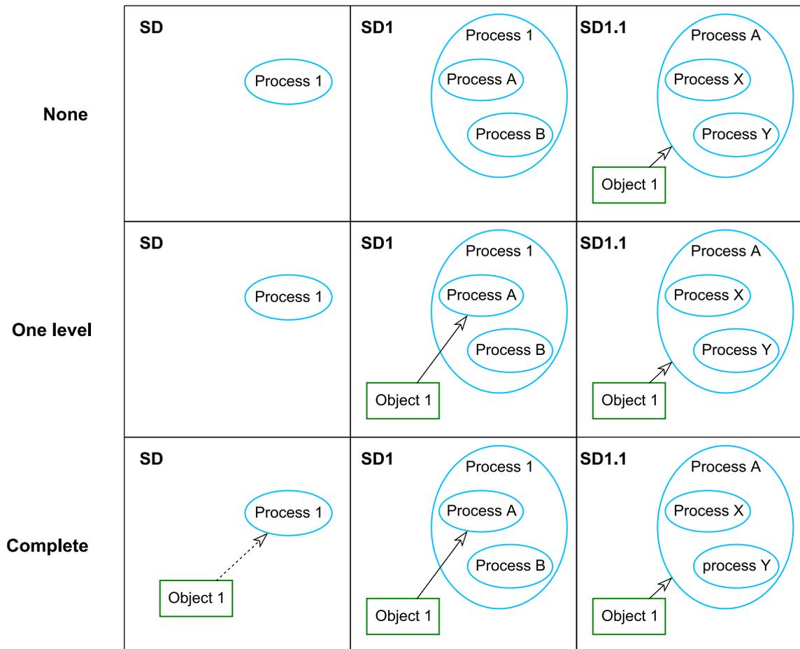
Figure 5.4: Comparison of effects on diagrams of the three modes of propagation: **None**, **One level** and **Complete**. The state of the each row is different after connecting the **Object 1** in the third diagram.
