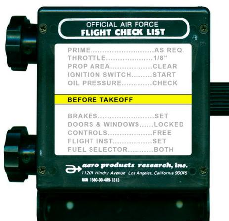
Figure 3.9: C-46 Commando aircraft scroll checklist<sup>11</sup>.
