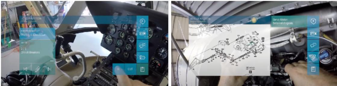
Figure 3.4: Atheer's AiR Enterprise is used to inspect a helicopter<sup>6</sup>.
