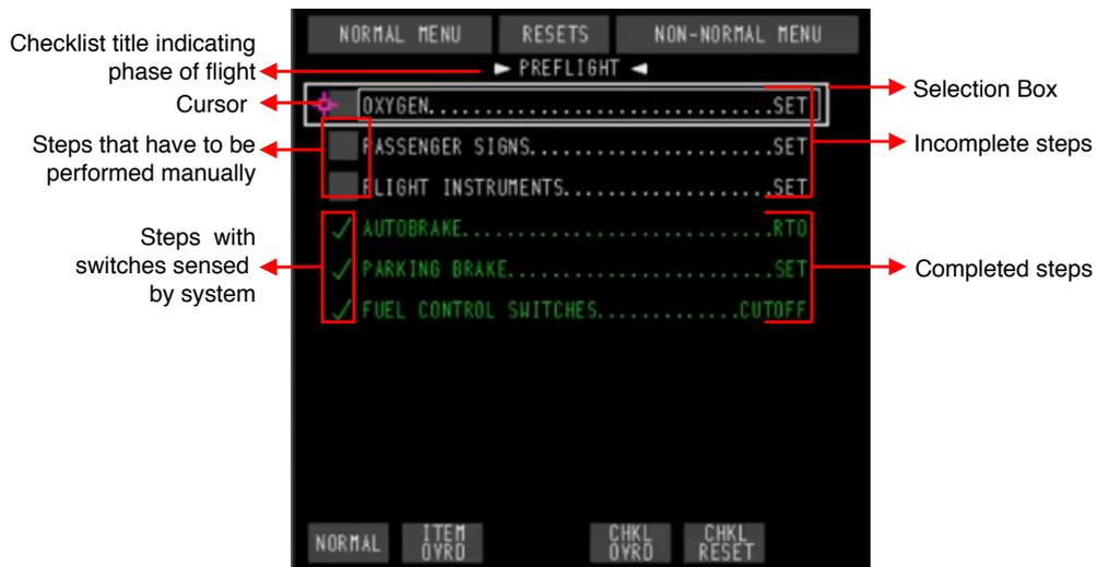
Figure 4.4: Pre-flight checklist related to normal procedures<sup>6</sup>.
