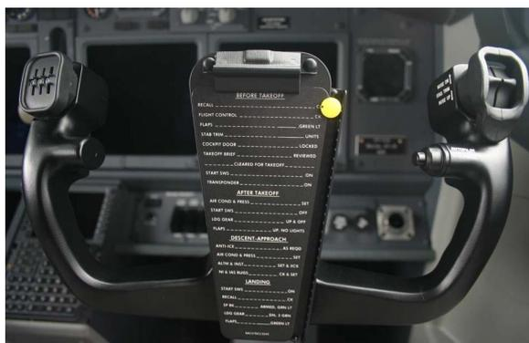
Figure 3.8: Checklist attached to yoke in Boeing 737<sup>10</sup>.
