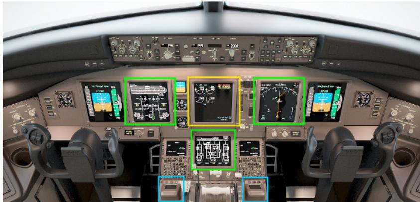
Figure 4.2: Boeing 777 flight deck layout<sup>4</sup>.
