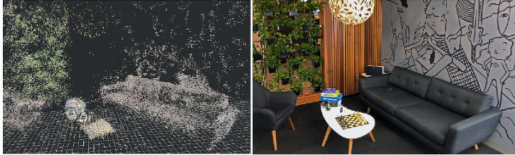
Figure 6.2: Left: Visualized accumulated frames of mapped real world with found tracked feature points<sup>2</sup>. Right: Real world environment<sup>2</sup>.
