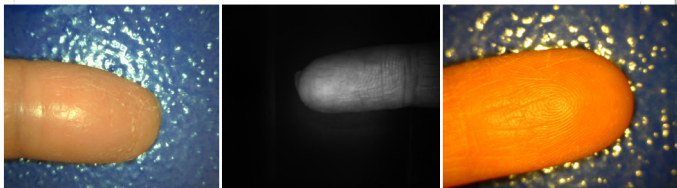
Figure: The surrounding light impact on fingerprint image
