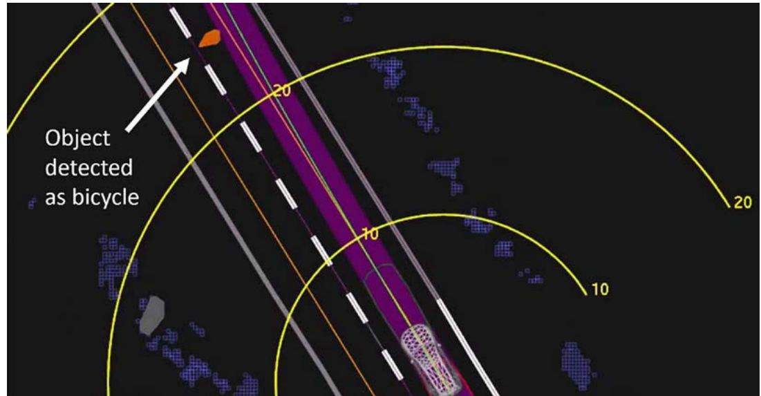
Figure 3 View of the self-driving system data playback at about 1.3 seconds before impact, when the system determined an emergency braking maneuver would be needed to mitigate a collision. Yellow bands are shown in meters ahead. Orange lines show the center of mapped travel lanes. The purple shaded area shows the path the vehicle traveled, with the green line showing the center of that path.
