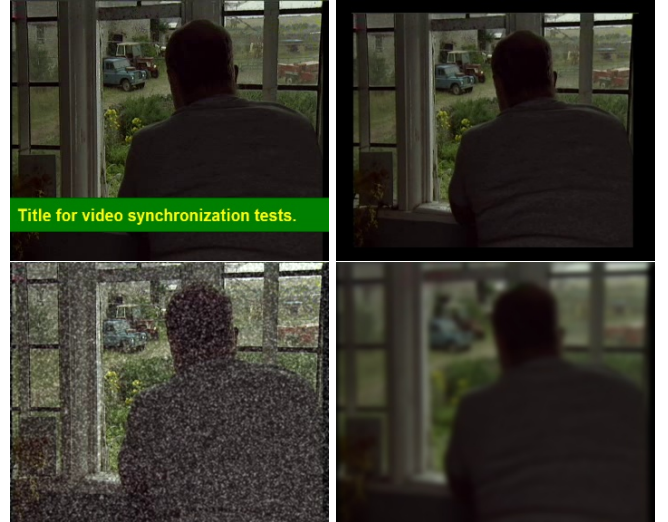
Fig. 5. Examples of video distortions (top - overlaid banner, 90% resize; bottom - 30% noise, blur with \sigma = 3.0 ).
