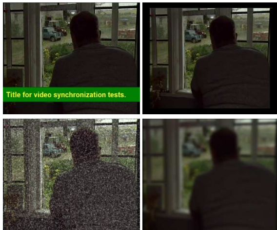
Figure 4. Examples of video distortions ( top – overlaid banner, 90% resize; bottom – 30% noise, smooth with \sigma 3.0).
