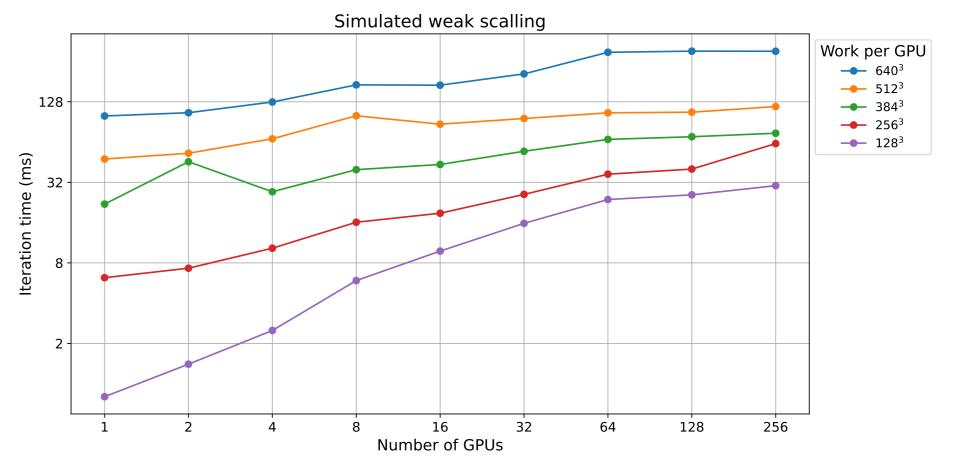
We run the simulation across multiple GPUs, allowing users to specify how the domain is divided and each subdomain assigned to a specific GPU. Each subdomain can operate with its own spatial and temporal resolution.
