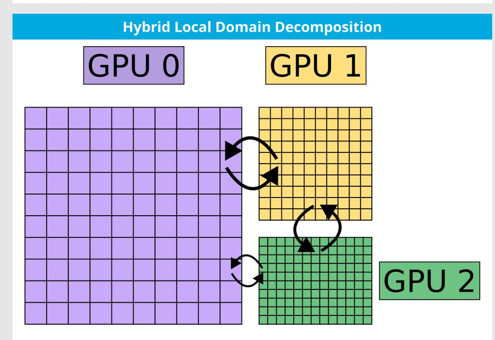
The simulation speed was tested on domains ranging in size from 128<sup>3</sup> to 4096<sup>3</sup> grid points, using a uniform 3D decomposition across up to 256 GPUs on the Karolina supercomputer, with all subdomains maintaining the same resolution. The strong scaling graph indicates substantial speedup for sufficiently large domains.
