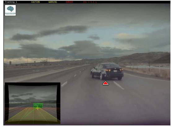
Fig. 3. Visualization of the collision warning. The bottom left picture shows rectified image with predicted object track. The top bar shows the signals issued by the system.
