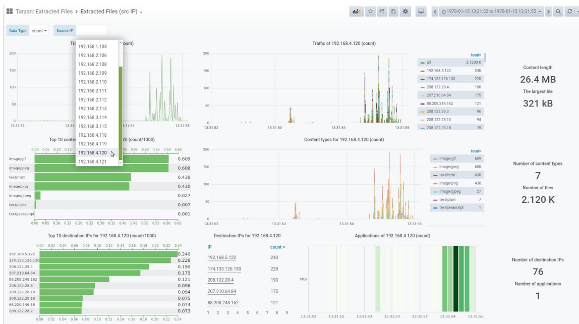
Figure 4.13: An example of the dashboard presenting data regarding extracted files for the specific source IP address (192.168.2.120).
