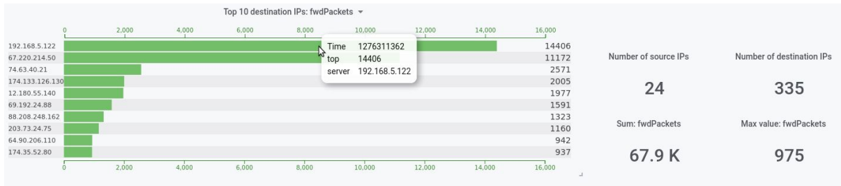
Figure 4.7: Example of the top statistics of destination IP addresses using bar chart (left) and overall indicators (right) representing numbers of (source and destination) IP addresses, summary and maximum value of the data series. Charts are synchronized with the time range filter.
