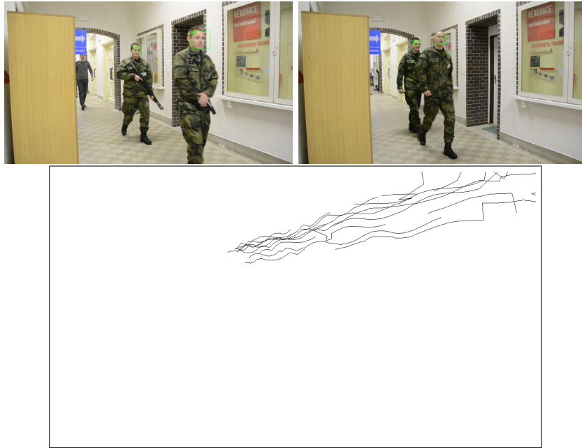
Figure 9: Face detection module. Two example frames from the input video and the resulting trajectories.
