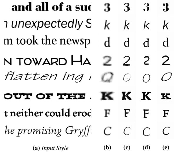
Figure 7: Effects of various parts of the architecture. (b) is the forward network without a discriminator; (c) is the GAN with a discriminator that does not see the input style; (d) is the network with GAN looking at style; and (e) is the larger, final network. Note that the pre-gan results may be convincing, but blurry.
