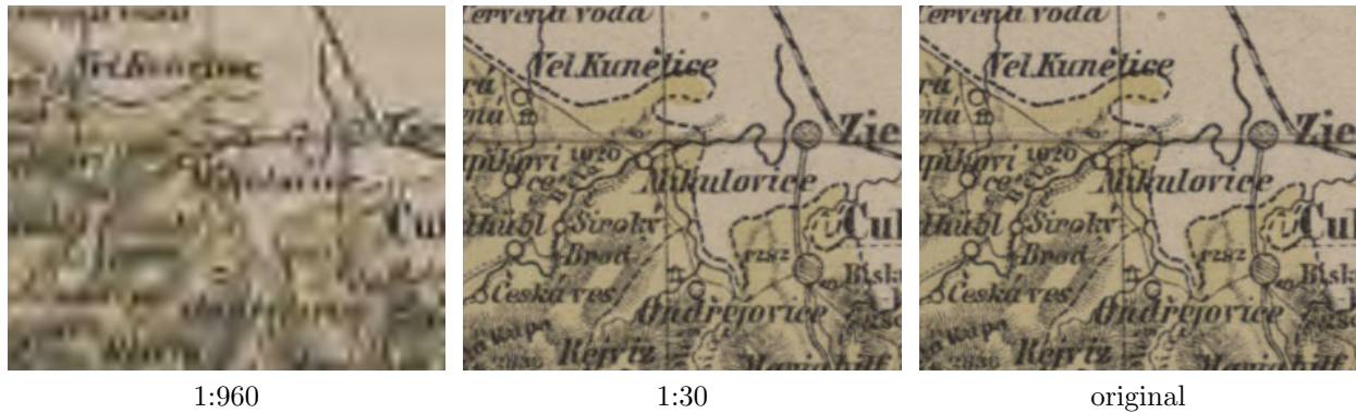
Figure 10: Visual image quality comparison on detail view. Cropped from a larger image. Observe compression artefacts. At first glance, the image with the 1:30 compression ratio is indistinguishable from the original. But when you look at this image in more detail, you may notice some inconspicuous artifacts even here.
