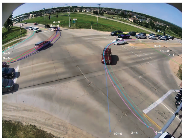
Figure 1. The main idea of this task — counting vehicles for every pre-defined movement of interest (travel direction).
