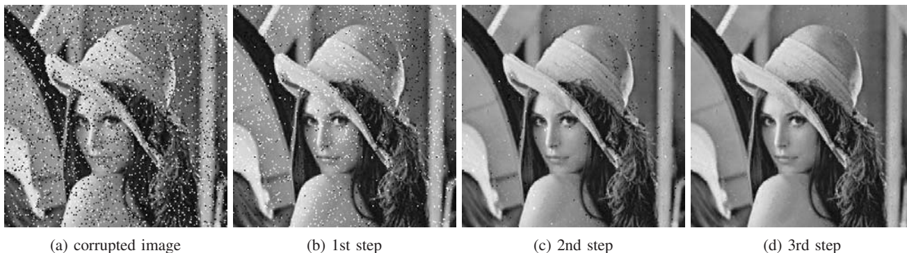
Fig. 5: Demonstration of filtering 10% noise from the training image by one of the best evolved filters in 3 CA steps.
