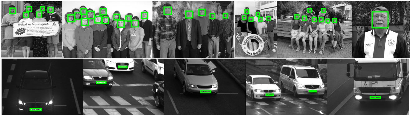
Fig. 9. Examples of detected objects on selected images from testing datasets for face detection (top) and license plate detection (bottom).
