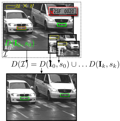
Fig. 2. (top) The detection process on pyramidal image representation \mathcal{I} . The detection window of size u \times v (yellow), is used for classification of every position m, n in image (example in red). The result of detection on each image is a set of locations D(\mathbf{I}, s) accepted by the classifier (green). (bottom) The final detection result after non-maxima suppression.
