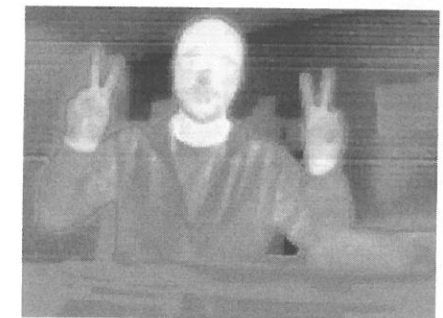
Illustration 6 (colored). Lepton 3 video frame captured by v4l2lepton3 in RGB888 format colored using fusion palette after internal histogram image normalization
