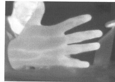
Illustration 5. Lepton 3 video frame captured by v4l2lepton3 in raw Y14 format after linear normalization
