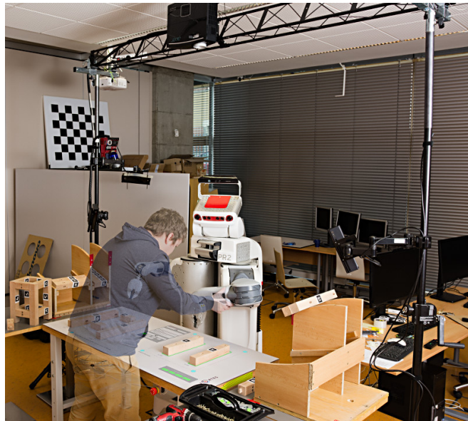
Fig. 1. Setup of the novel interactive system concept where all the interaction elements (visualization and control) are gathered in a shared workspace (example of setting program parameters using a robotic arm and gestures; image edited).
