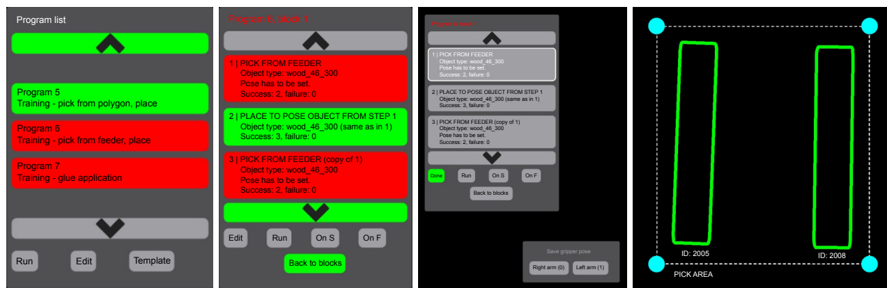
(a) List of programs. Green ones are ready to run, red ones need to set parameters. (b) List of instructions. Green ones are ready to run, red ones need to set parameters. (c) A small dialog shows if the robot is able to detect an object in the feeder and allows the user to save the arm pose. (d) Polygon defining the area on the table from which the objects will be picked up. The green outlines correspond to detected objects.
