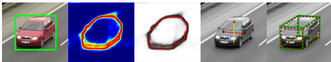
Fig. 6. Estimation of 3D bounding box. Left to right: image with vehicle 2D bounding box, output of contour object detector [67], our constructed contour, estimated directions towards vanishing points, ground truth (green) and estimated (red) 3D bounding box.
