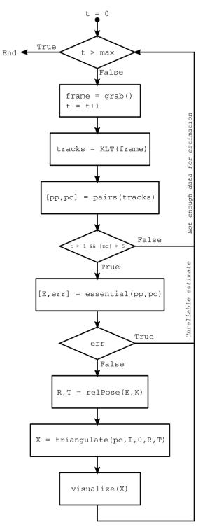
Control flow of KLT version of SFM as implemented in sfmKLT.m. KLT() is implemented by PointTracks class which take care of correct tracking of features and for each feature provide its movement history. Pairs are selected by constructEndpoints(). Essential matrix and relative pose are solved by internal Matlab functions which runs RANSAC (MSAC actually) with 5-point algorithm and selects most probably R,T.
