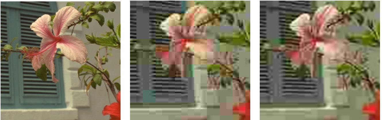
Figure 10: Visual comparison of the original image (left), DCT (middle, PSNR 23.0 dB), and LCT (right, PSNR 23.3 dB).
