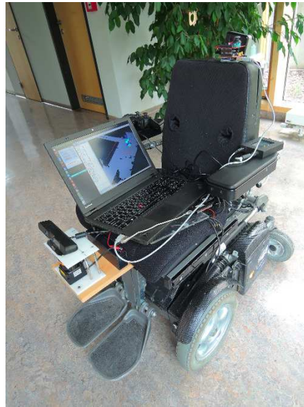
Figure 1: The C400 permobil wheelchair equipped with a control command communication interface and with a scanning laser and a RGB-D sensors.
