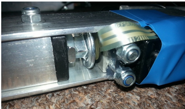
Fig. 8. Force-sensitive resistors placement. The inner profile is movable in digits of singles a millimeter. This ensures perfect functionality of the force-sensitive resistor.
