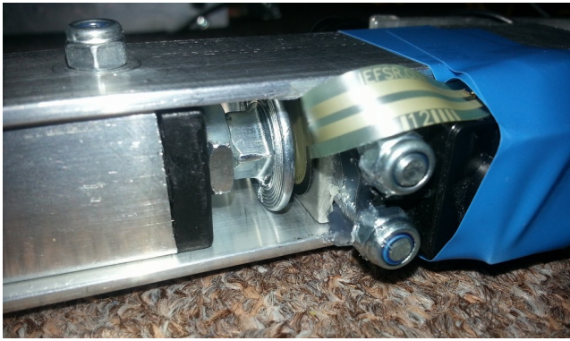
Fig. 3. Force-sensitive resistors placement. The inner profile is movable in digits of singles a millimeter. This ensures perfect functionality of the force-sensitive resistor.
