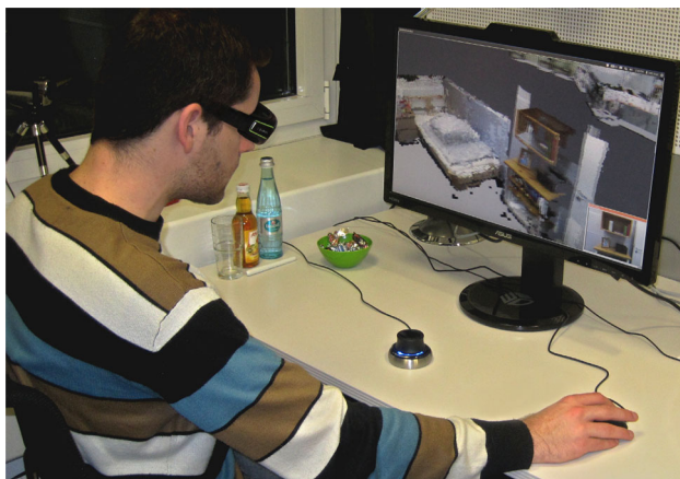
Fig. 9 Participant in front of user interface with stereo glasses, standard mouse, and SpaceNavigator 3D mouse
