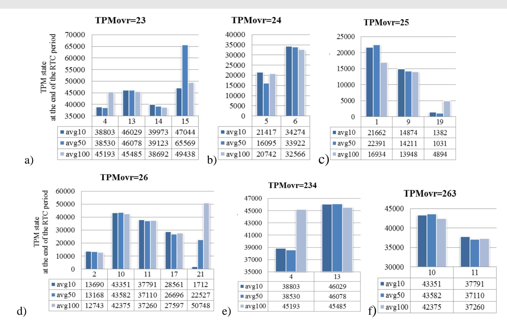
Devices with the same TPMovr value can be distinguished on basis of the TPMstate value – selected results for the RTCPS=13 (a-d) and for RTCPS=15 (e, f). avg10, avg50 and avg100 means the value was evaluated as a mean value value value was evaluated as a mean value val
