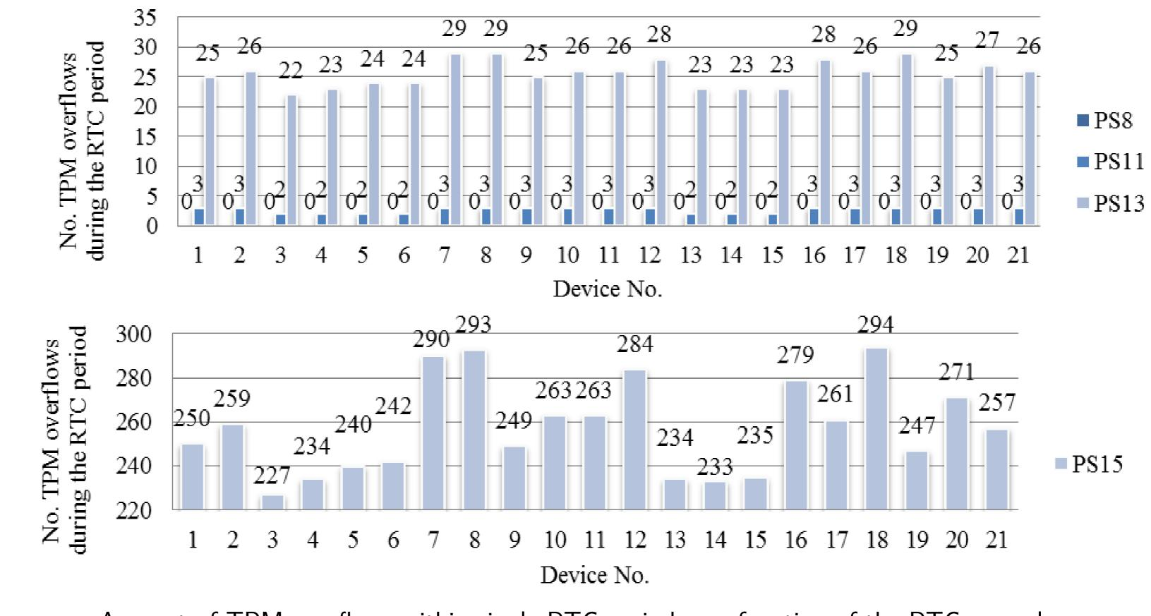
Amount of TPM overflows within single RTC period as a function of the RTC prescaler.
