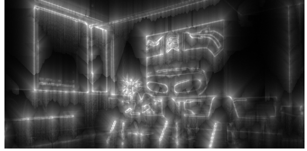
Figure 8: Application of the Sobel operator and IDT to the image on Figure 1a
