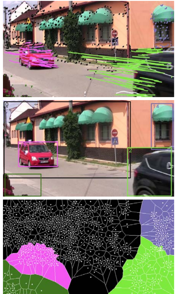
Figure 4. Motion segmentation of scene with two moving cars. From top: tracks, bounding boxes, Voronoi tessellation of the whole image.
