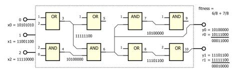
Fig. 3 Parallel simulation of a combinational circuit. The values  $y_0$  and  $y_1$  are the results of simulation;  $r_0$  and  $r_1$  are the required outputs
