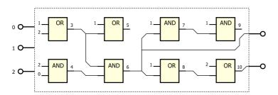
**Fig. 2** Example of a candidate circuit. CGP parameters are as follows: l = 3,  $n_c = 4$ ,  $n_i = 3$ ,  $n_o = 2$ ,  $n_r = 2$ ,  $\Gamma = \{AND (0), OR (1)\}$ . Nodes 5,7 and 9 are not utilized. Chromosome: 1,2,1, 2,0,0, 1,3,1, 3,4,0 1,6,0, 1,6,1, 1,7,0, 2,8,1, 6, 10. The last two integers indicate the outputs of circuit. The function of a gate is typed in bold.
