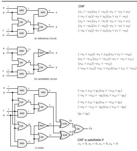
Fig. 5 Example of transformation of reference circuit, candidate circuit and miter to CNF
