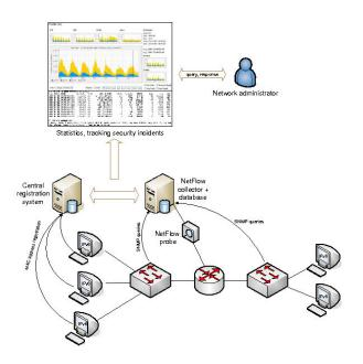
Fig. 2. Integrated monitoring system for IPv4 and IPv6
