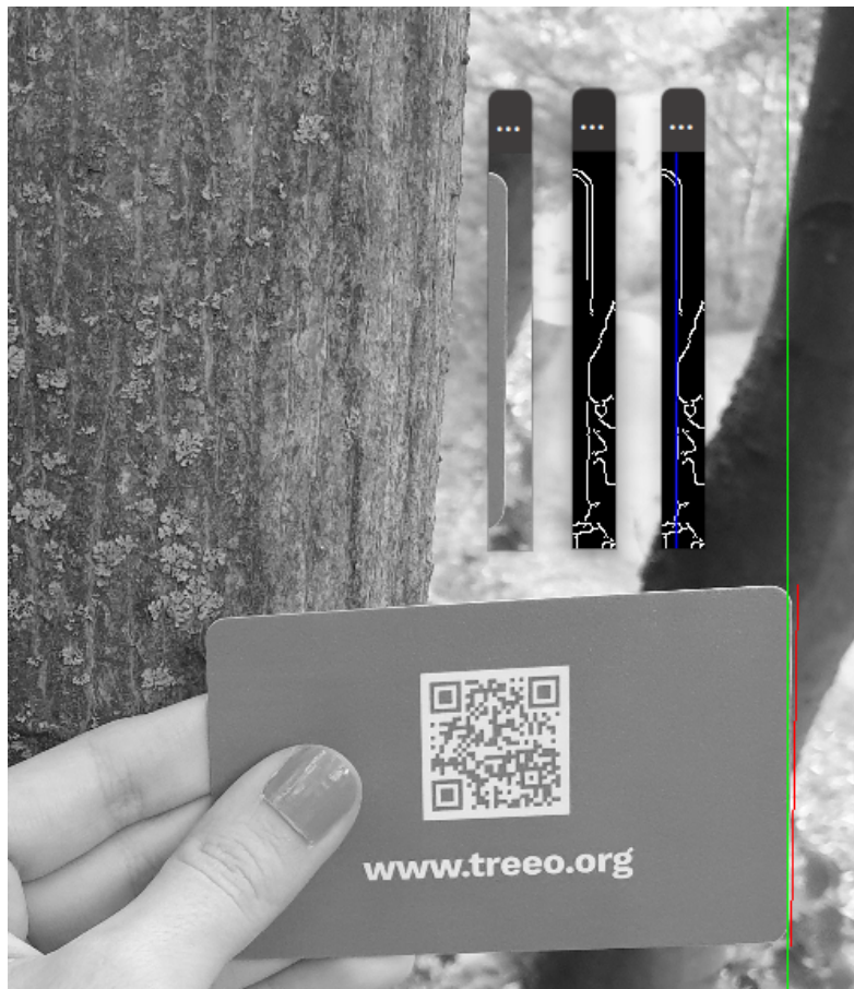
Example of refinement with Hough lines. Red line is the original edge found by SIFT, the green line is refined edge with our method. Neighborhood of this edge can be seen in the first cut out region, canny edge detection in second and line found by Hough transformation in the third region (blue line which is also green in the whole image).
