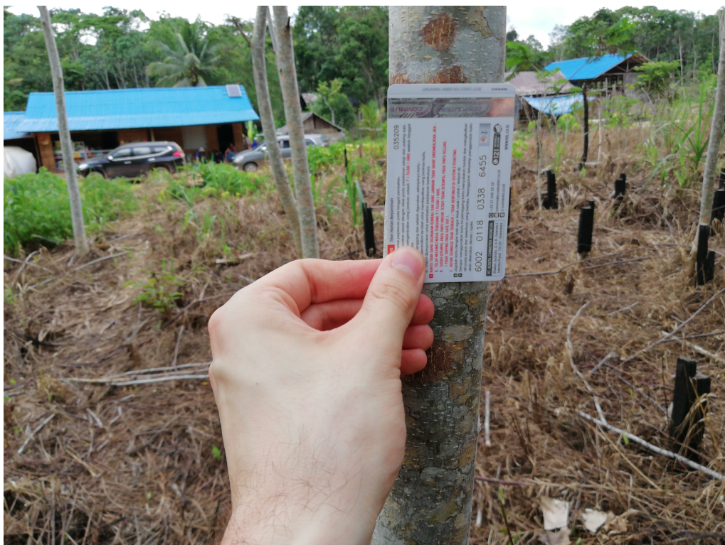
Example of the image with the tree-trunk and the known card to process DBH measurement.
