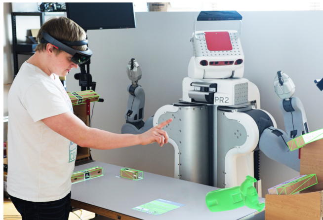
Fig. 1: Spectator’s view of the collaborative workspace, with projected user interface, extended by virtual objects seen through the HMD. Example of setting program parameters using the HMD gestures.
