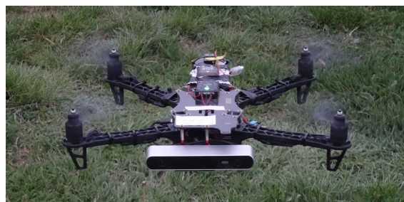
Figure 3: Test drone with Pixhawk control unit, ZED stereoscopic camera and Nvidia Jetson supercomputer, shot just above ground.
