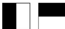
Figure 7: Haar wavelet filters that compute the responses in x (left) and y direction (right). The dark parts have weight -1 and the light parts +1 [1].
