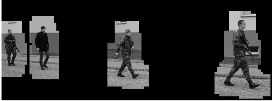
Figure 11: Masked areas of video frame where the motion using background subtraction technique was detected
