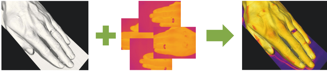
FIGURE 1: Visualizing the data fusion process: the 3D model from a 3D scanner (left) is combined with the 2D thermal images obtained using a thermal camera (middle) to produce the final 3D thermal model (right).
