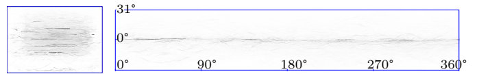
Figure 6: Edge accumulation. Left: Normalized average from all accumulated images. Right: Accumulated panorama image.
