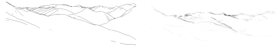
Figure B.10: Accumulation of matched edges for a single query image. We split the area around the GPS location of the query image uniformly into a grid of 9 \times 9 cells (resolution of 0.001^\circ in both N-S and W-E directions). From each cell we render synthetic silhouettes ( left ) and match them to edges in the query image. In the accumulated image, we increase the value of all pixels containing a synthetic silhouette, which contributed positively to the matching score. We run such an evaluation for every cell in the grid and sum up the accumulators to obtain one accumulated image for a query ( right ).
