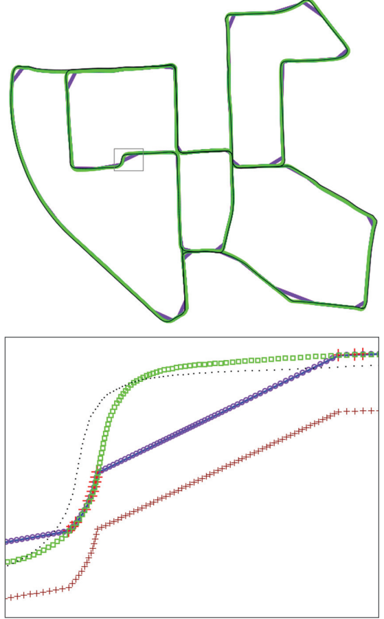
Fig. 4. Kitti00 trajectory compacted to only 355 poses out of 4541. v0 and v1 in violet, v2 in green, ground truth in black (top), a detailed view of the trajectory, optimized poses marked by large red crosses, v0 small dark red crosses (shifted vertically to not overlap with v1), v1 violet circles, v2 green rectangles, ground truth in black (bottom).
