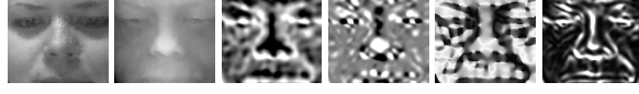
Figure 4: From left to right: texture, range image, mean curvature, Gaussian curvature, shape index, and eigencurvature.
