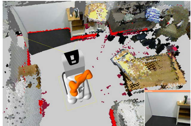
Fig. 6. The 3D mixed reality environment consisting of a robot model, 2D laser data, a 2D map, a combination of the live RGB-D data in current field of view of the robot (visualized using thin lines) and the 3D voxel-based map outside it and a video stream.
