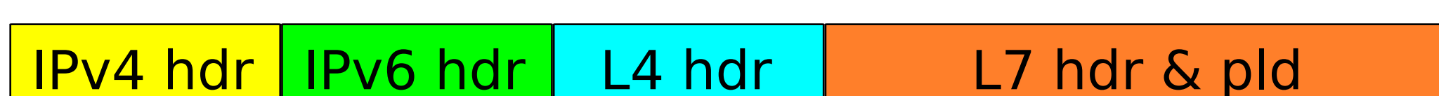
Figure 3: Encapsulation in 6to4 (RFC3056), 6rd (RFC5969), ISATAP (RFC5214) - IP protocol = 41
