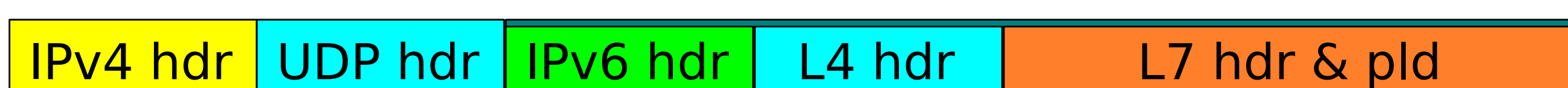
Figure 4: Encapsulation in Teredo (RFC4380) - arbitrary UDP port may be used
