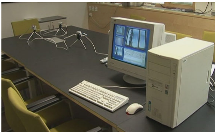
Figure 1: Online video editing system setup with three firewire cameras.
