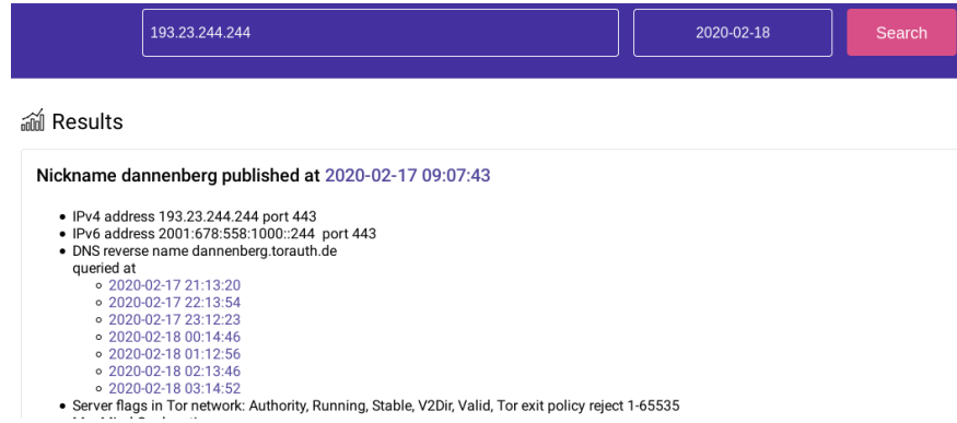
Fig. 1. A detective inserts an IP address and time into the tool to learn that the IP address was a part of the Tor network.
