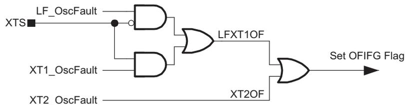
Figure 5-8. Oscillator-Fault Logic
