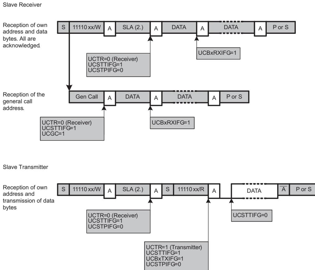
Figure 17-11. I<sup>2</sup>C Slave 10-bit Addressing Mode
