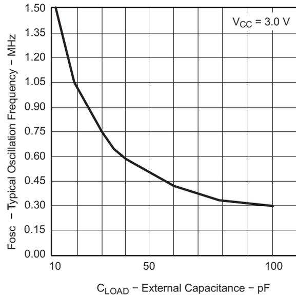
**Figure 8-2. Typical Pin-Oscillation Frequency**
