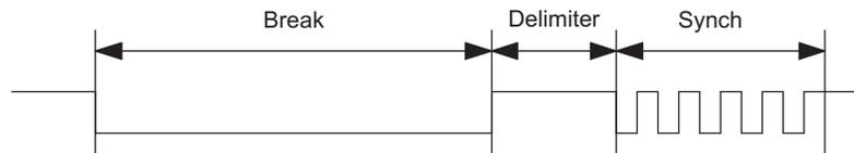
Figure 15-5. Auto Baud Rate Detection - Break/Synch Sequence
