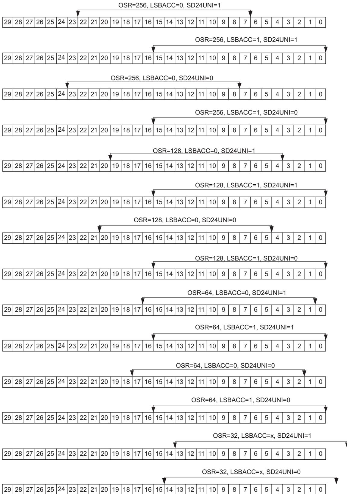
Figure 27-5. Used Bits of Digital Filter Output
