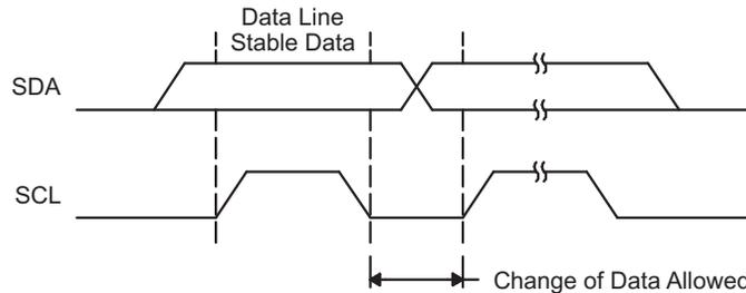
Figure 17-4. Bit Transfer on the I<sup>2</sup>C Bus
