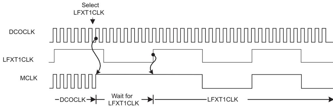
**Figure 5-9. Switch MCLK from DCOCLK to LFXT1CLK**
