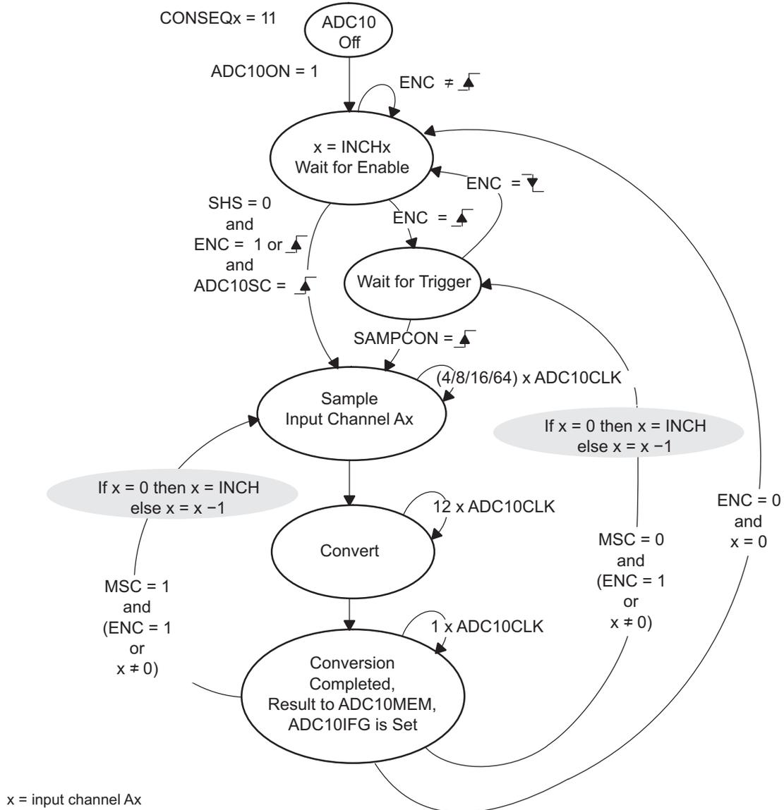
Figure 22-8. Repeat-Sequence-of-Channels Mode
