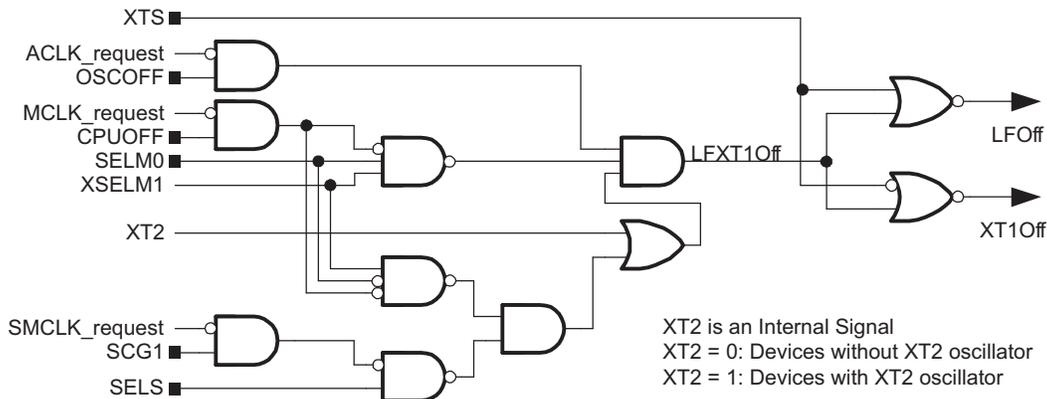
**Figure 5-3. Off Signals for the LFXT1 Oscillator**
