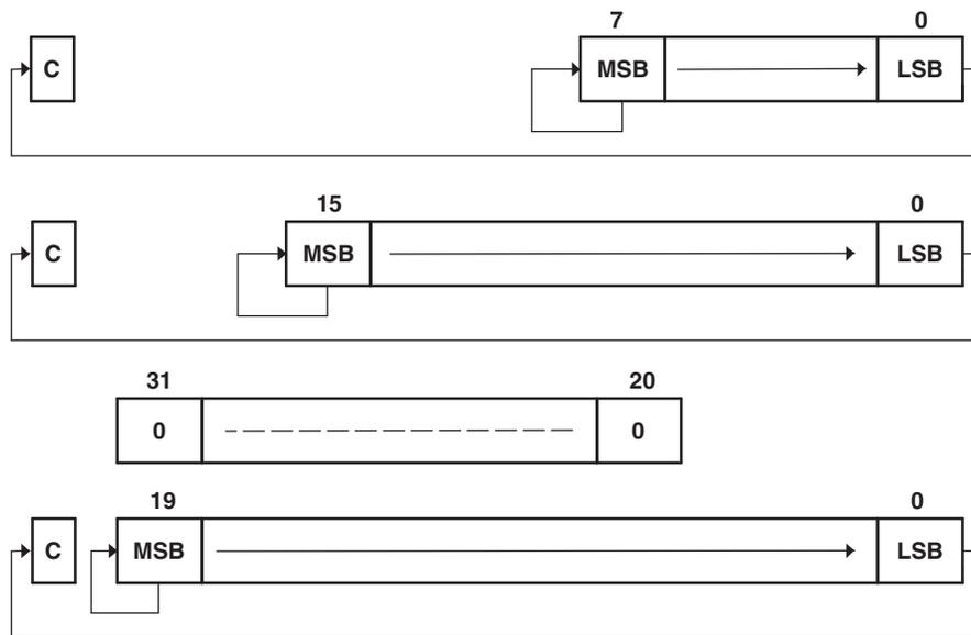
**Figure 4-48. Rotate Right Arithmetically RRAX(B,A) – Non-Register Mode**
