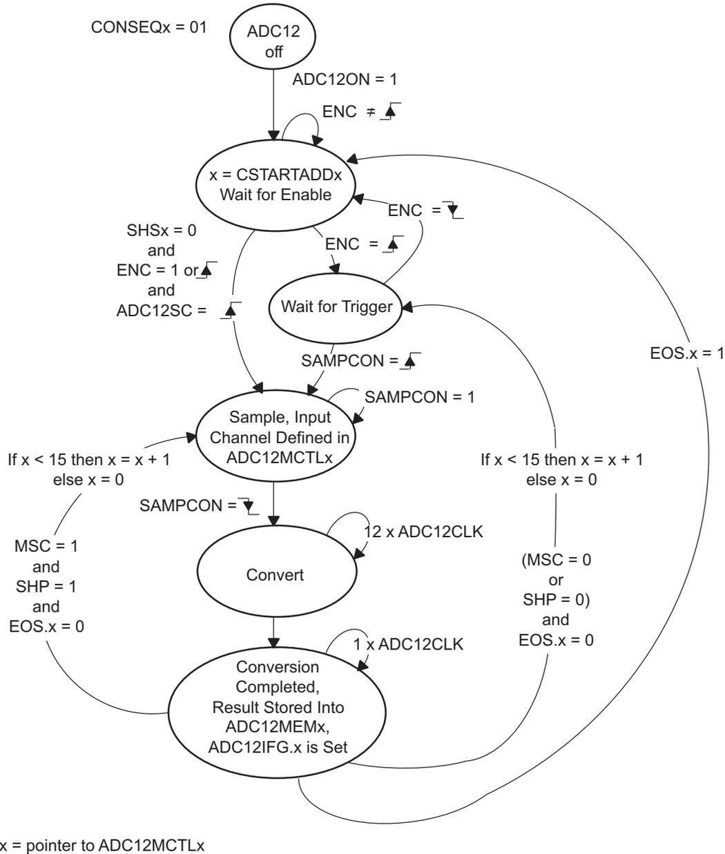
Figure 23-7. Sequence-of-Channels Mode
