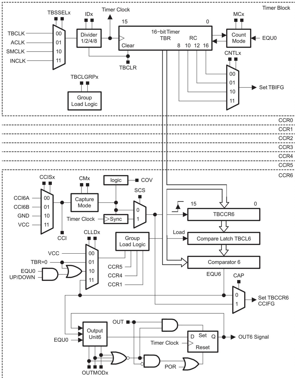
NOTE: INCLK is device-specific, often assigned to the inverted TBCLK, refer to device-specific data sheet.
