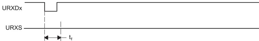
**Figure 15-8. Glitch Suppression, USCI Receive Not Started**
