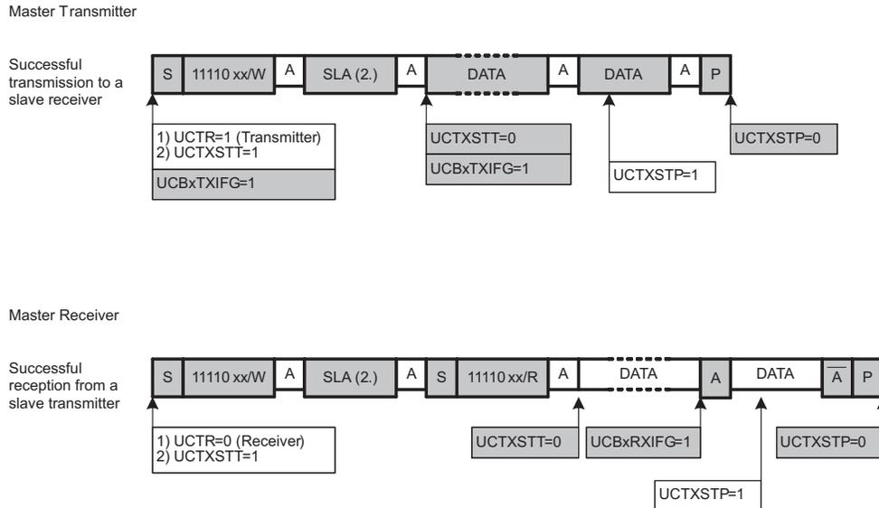
Figure 17-14. I<sup>2</sup>C Master 10-bit Addressing Mode
