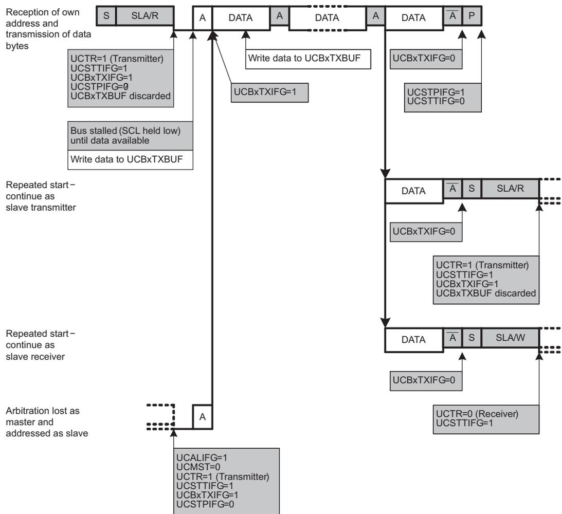
Figure 17-9. I<sup>2</sup>C Slave Transmitter Mode
