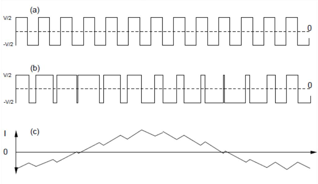
Figure 2. Waveforms in PWM inverter: (a) Unmodulated carrier; (b) Modulated carrier; (c) Current in inductive load
