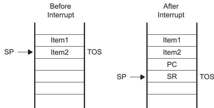
**Figure 2-6. Interrupt Processing**
