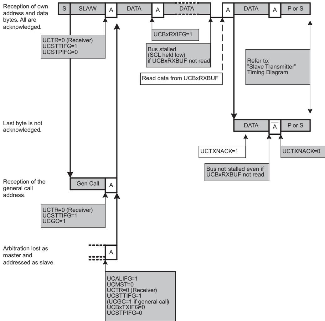
Figure 17-10. I<sup>2</sup>C Slave Receiver Mode
