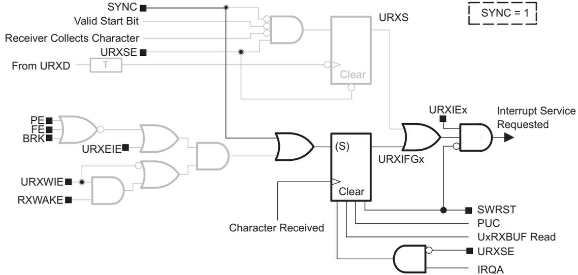
Figure 19-11. Receive Interrupt Operation
