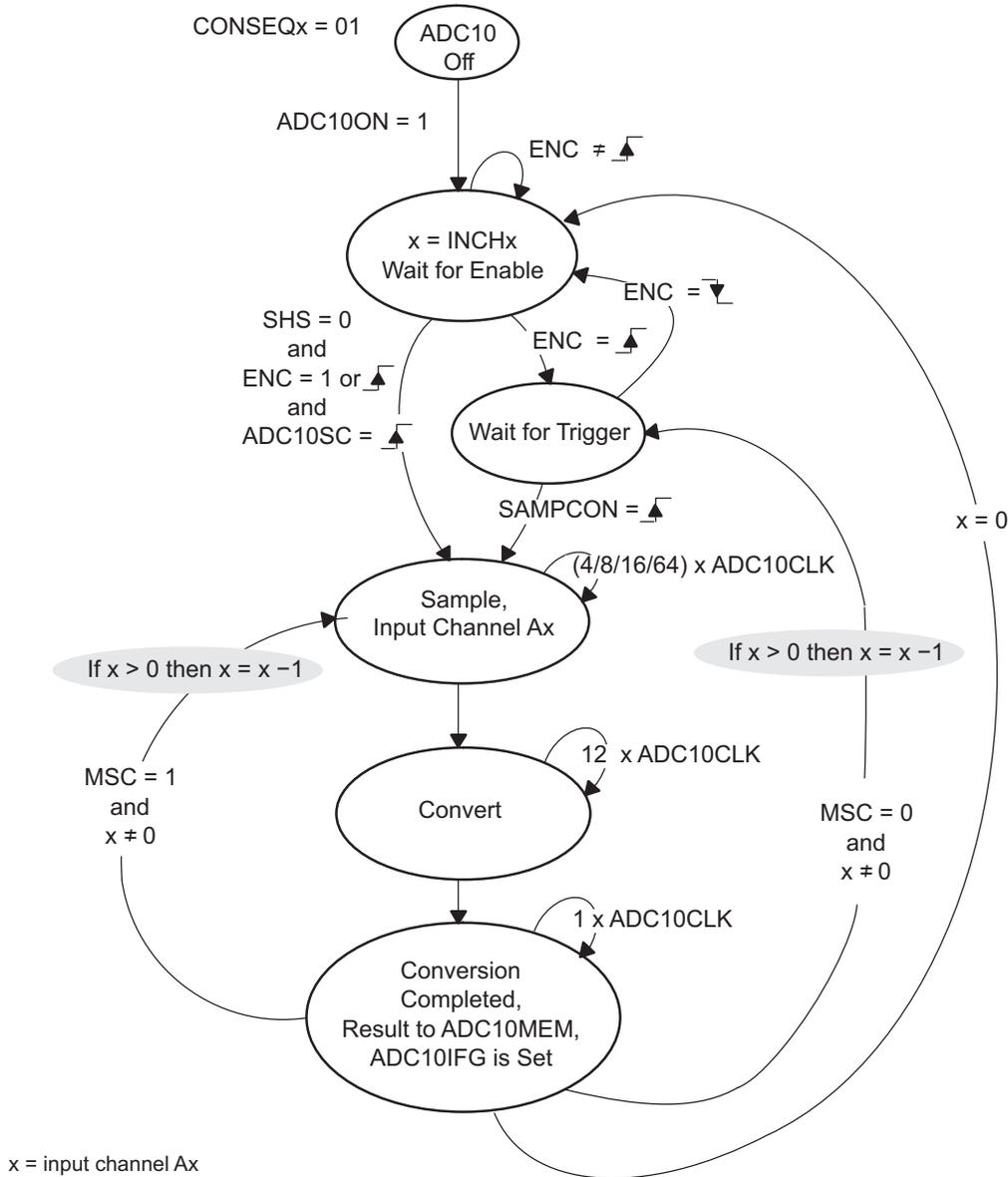
Figure 22-6. Sequence-of-Channels Mode
