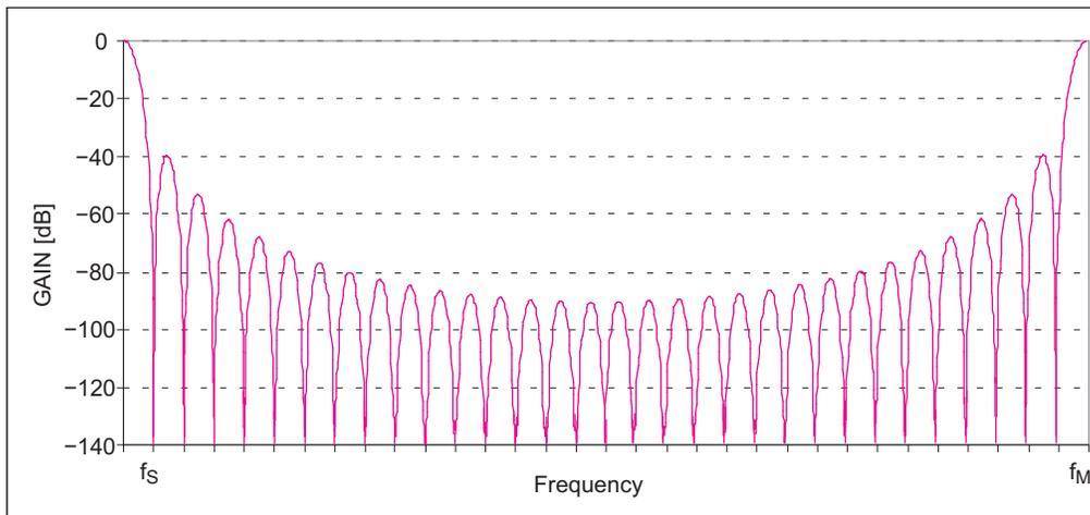
Figure 27-3. Comb Filter Frequency Response With OSR = 32
