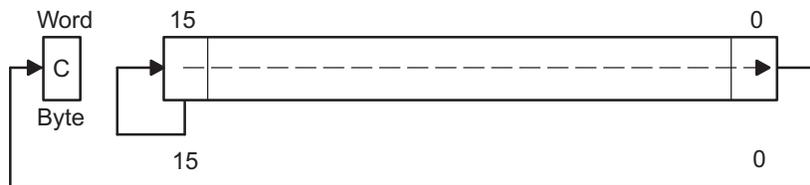
**Figure 3-17. Destination Operand – Arithmetic Right Shift**
