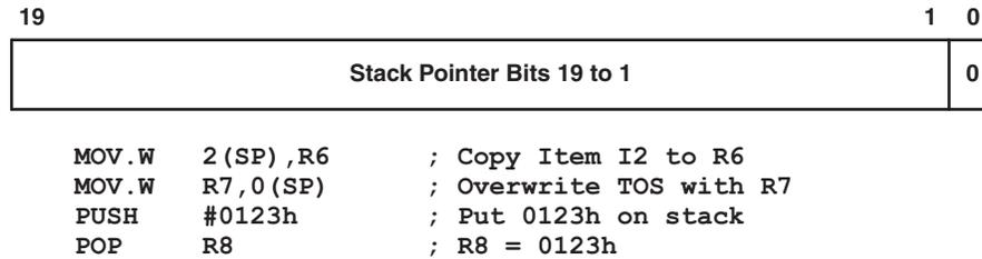
Figure 4-5. Stack Pointer
