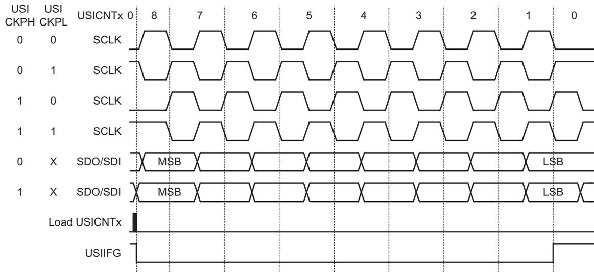
Figure 14-3. SPI Timing
