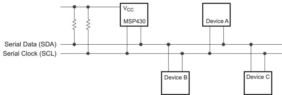
**Figure 17-2. I<sup>2</sup>C Bus Connection Diagram**
