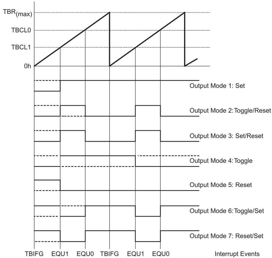
**Figure 13-13. Output Example, Timer in Continuous Mode**
