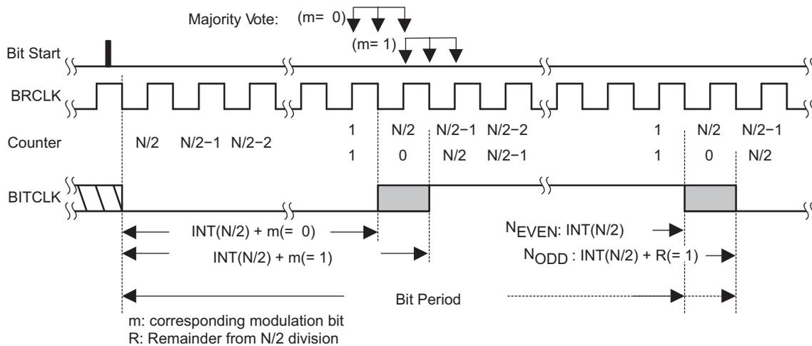
Figure 15-10. BITCLK Baud Rate Timing With UCOS16 = 0
