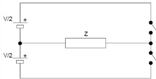
Figure 1. Half Bridge Switching Circuit
