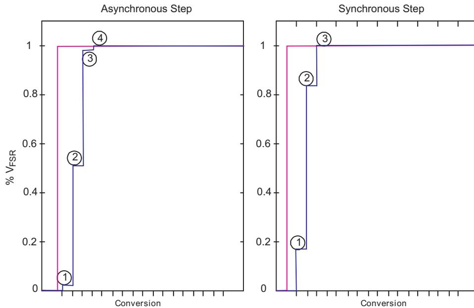
Figure 26-4. Digital Filter Step Response and Conversion Points
