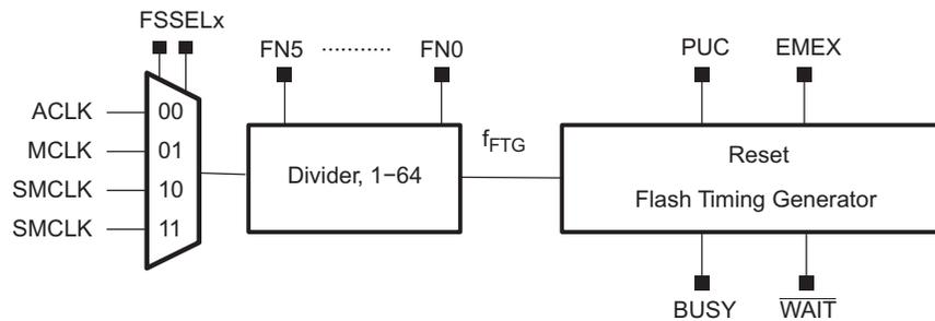
Figure 7-3. Flash Memory Timing Generator Block Diagram
