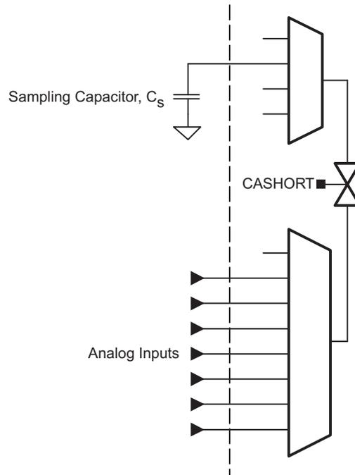
**Figure 21-2. Comparator\_A+ Sample-And-Hold**
