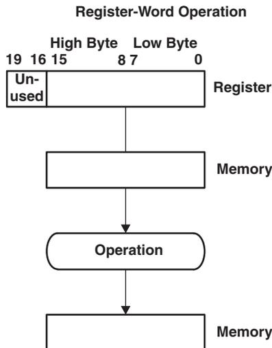
Figure 4-11. Register-Word Operation
