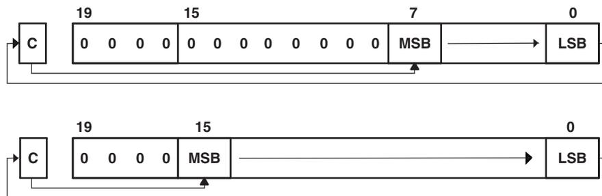
**Figure 4-40. Rotate Right Through Carry RRC.B and RRC.W**
