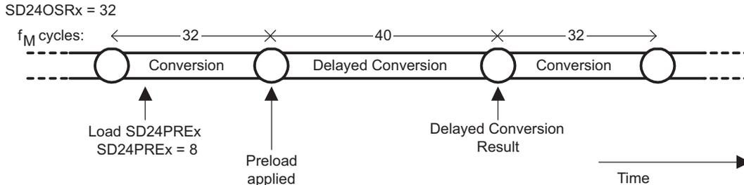
Figure 27-9. Conversion Delay Using Preload - Example
