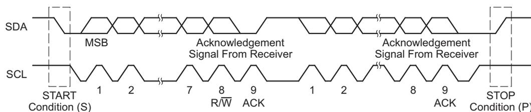
**Figure 17-3. I<sup>2</sup>C Module Data Transfer**
