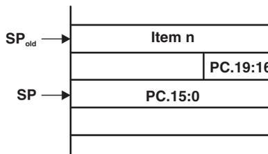
Figure 4-4. PC Storage on the Stack for CALLA
