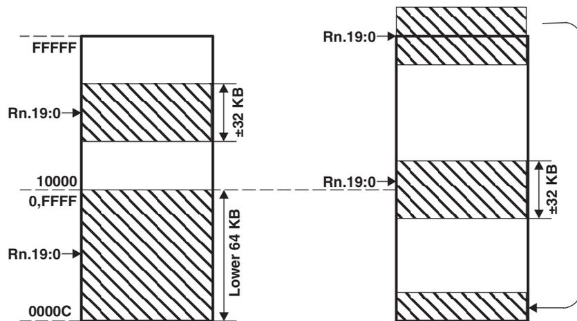
**Figure 4-17. Overflow and Underflow for Indexed Mode**
