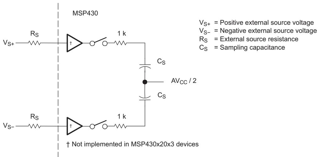
**Figure 26-2. Analog Input Equivalent Circuit**
