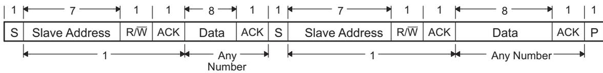
**Figure 17-7. I<sup>2</sup>C Module Addressing Format with Repeated START Condition**
