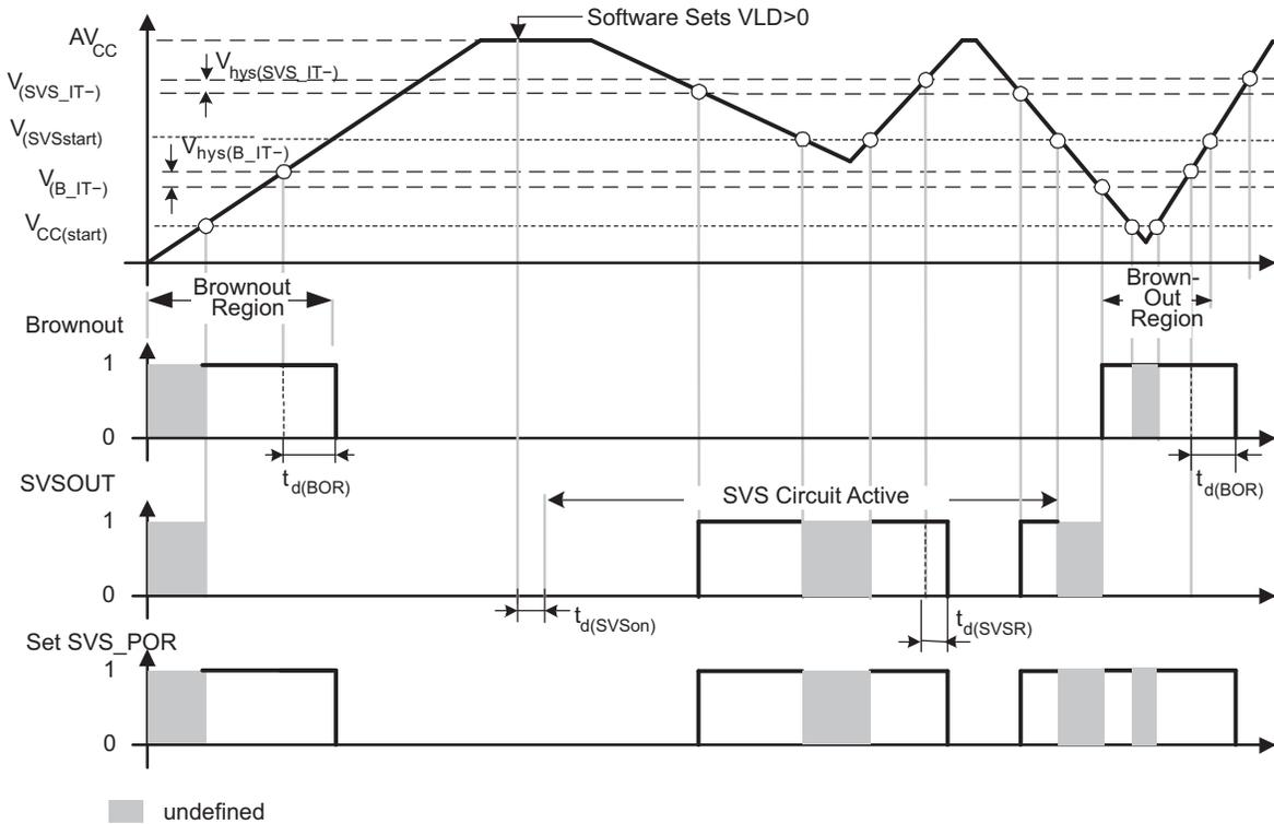
Figure 9-2. Operating Levels for SVS and Brownout/Reset Circuit
