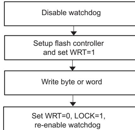
**Figure 7-8. Initiating a Byte/Word Write from Flash**
