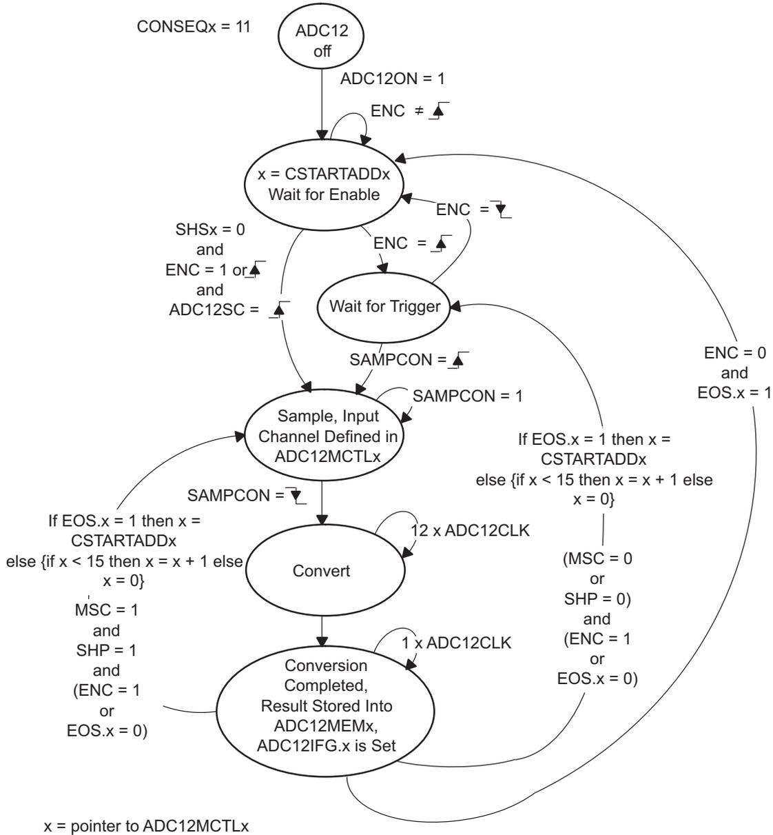
Figure 23-9. Repeat-Sequence-of-Channels Mode
