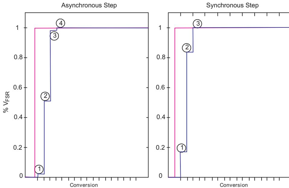
Figure 27-4. Digital Filter Step Response and Conversion Points
