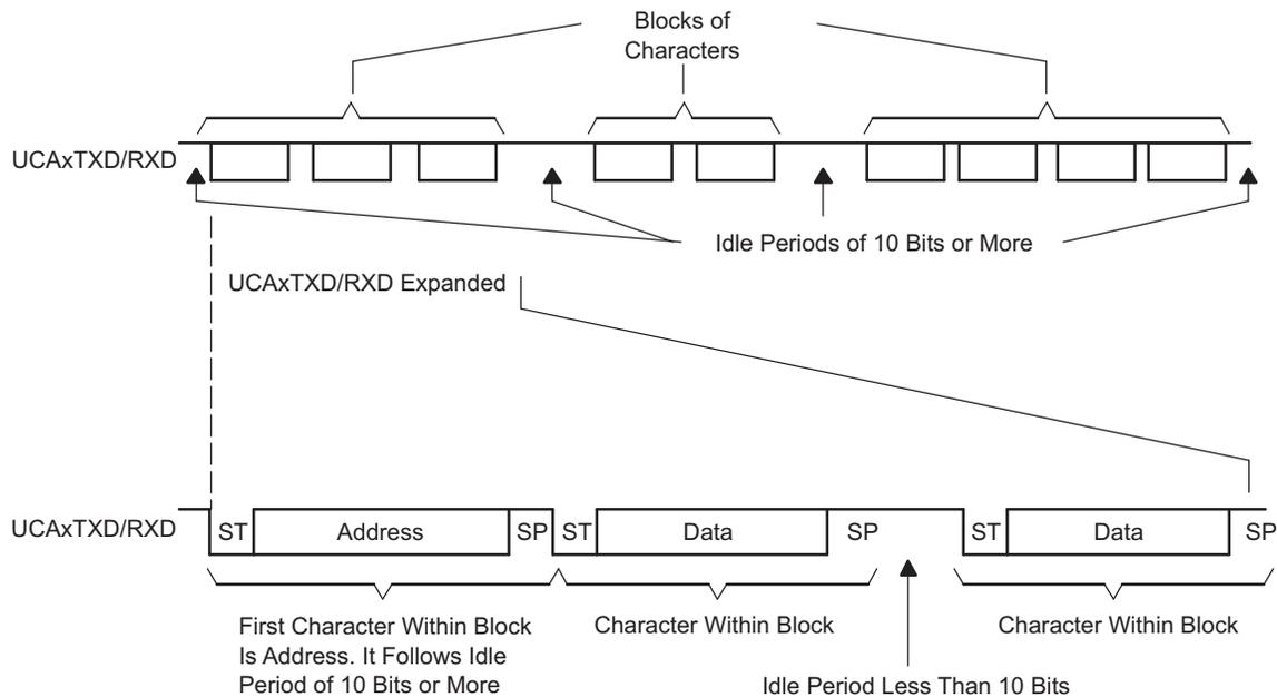
**Figure 15-3. Idle-Line Format**
