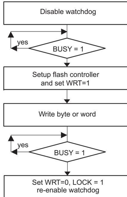
**Figure 7-9. Initiating a Byte/Word Write from RAM**
