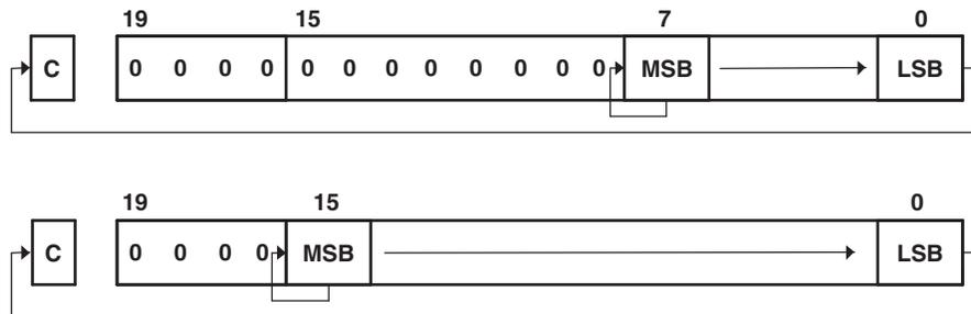
**Figure 4-39. Rotate Right Arithmetically RRA.B and RRA.W**
