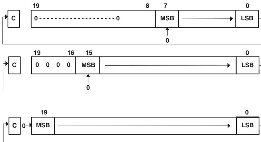
Figure 4-53. Rotate Right Unsigned RRUX(.B,.A) – Register Mode
