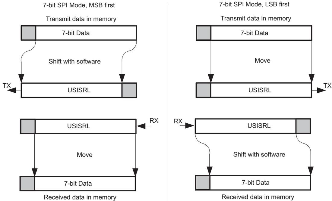
Figure 14-4. Data Adjustments for 7-Bit SPI Data
