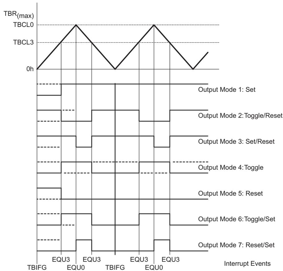
**Figure 13-14. Output Example, Timer in Up/Down Mode**
