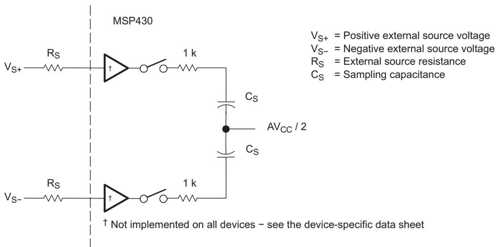
**Figure 27-2. Analog Input Equivalent Circuit**
