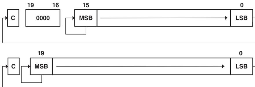
Figure 4-46. Rotate Right Arithmetically RRAM.[W] and RRAM.A
