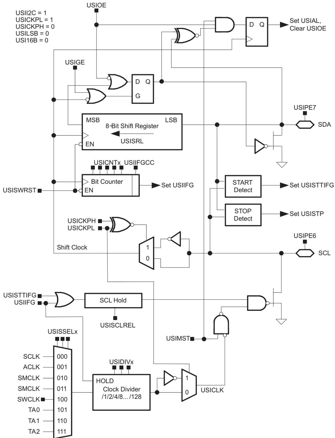
Figure 14-2. USI Block Diagram: I<sup>2</sup>C Mode
