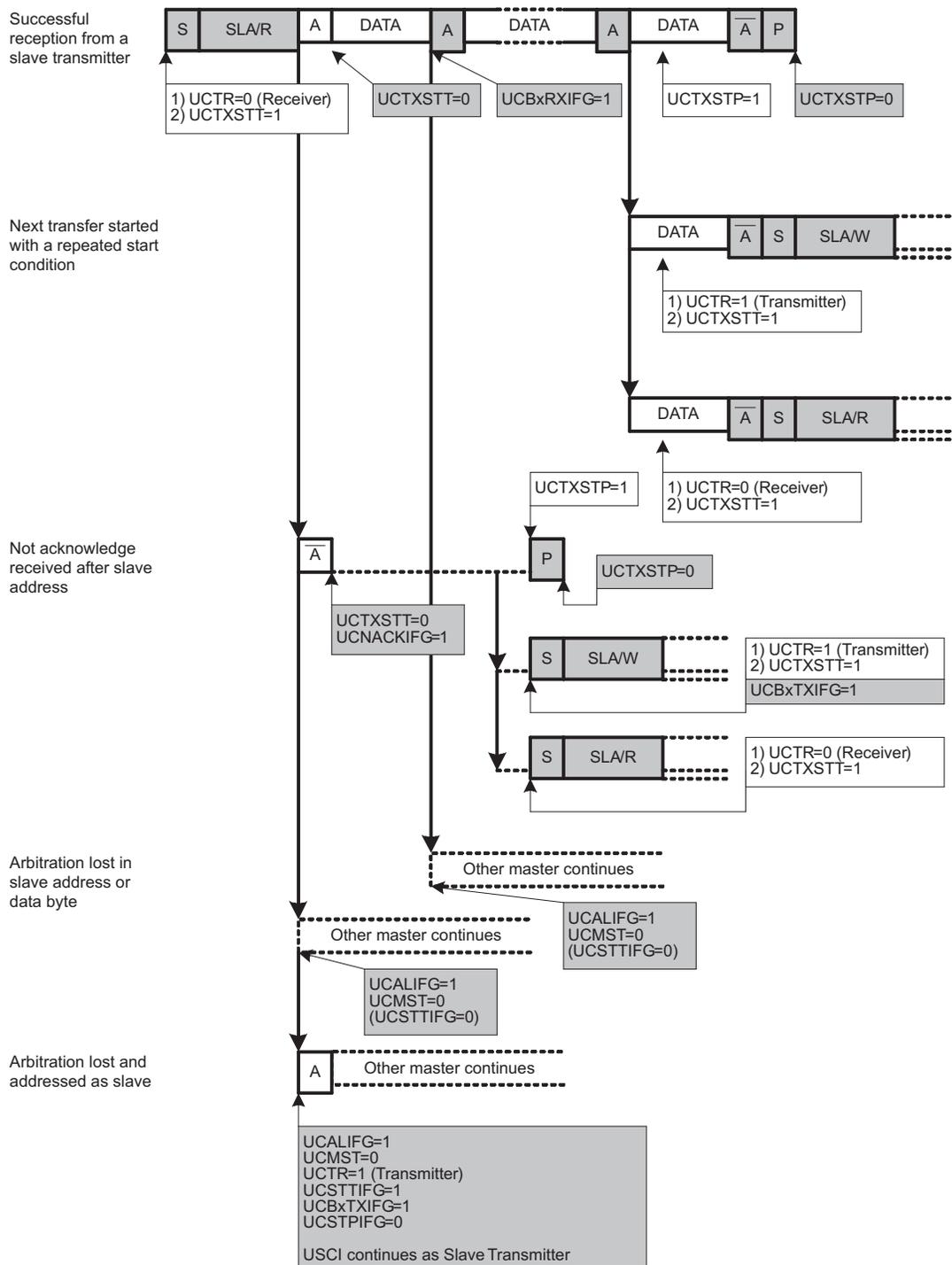
Figure 17-13. I<sup>2</sup>C Master Receiver Mode
